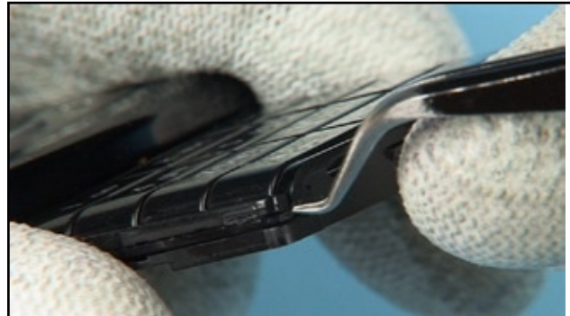
18. Insert the angled tweezers into the recess as shown.
